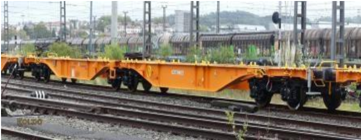
Figure 4: Wagon-plateforme type MMQ
